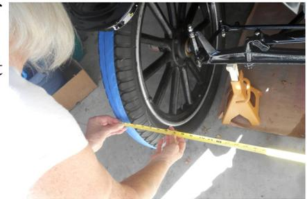
Set the end of the tape in the center of the mark.
