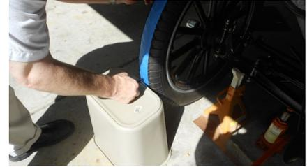
With a marker apply a mark completely around the tire on each wheel.
