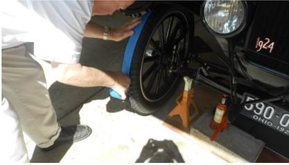
Apply tape completely around the tire.
