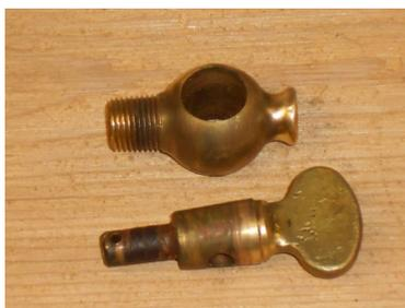
The beveled surface is grooved and corroded thus allowing gas to leak. Same happens to radiator petcocks.
