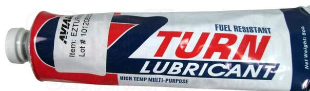
Last and most important get a tube of EZ Turn by United. It is an aviation lubricant that is heat and gasoline resistant. It doesn't harden or dry-out and provides an anti-seize agent. Put a thin coating over the entire surface of the stem keeping the hole clean and clear of debris. Once reassembled, a lite tap with a rubber mallet should put the last seal in place. EZ Turn is very sticky and hard to get off your fingers. Use a glove to apply.
