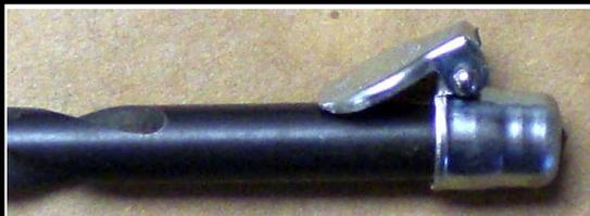
Flip up cap and insert drill bit. (Hint) Grind the drill bit tip flat to clean the oiler seat to the bottom.
