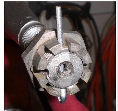
Bend the split ends of the Cotter Pin so that one is wrapped over the nut and the other is over the shaft or bolt end. This is what a properly installed Cotter Pin should look like.
