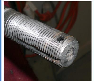
The bolt or shaft that corresponds to the pin and nut must have a hole drilled in it. Make sure the hole is clean and has the same diameter as the Cotter Pin.
