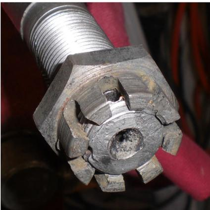
The Cotter Pin must be long enough to wrap over the nut and bolt end. Insert the Cotter Pin all the way into the hole so the loop fits snugly in the notch of the nut. You can cut off the excess, but you can not make it longer.
